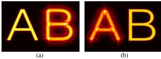
Figure 3. Accommodation effect of reconstructed image in complex modulation with focus on alphabet (a) 'A' and (b) 'B'.
