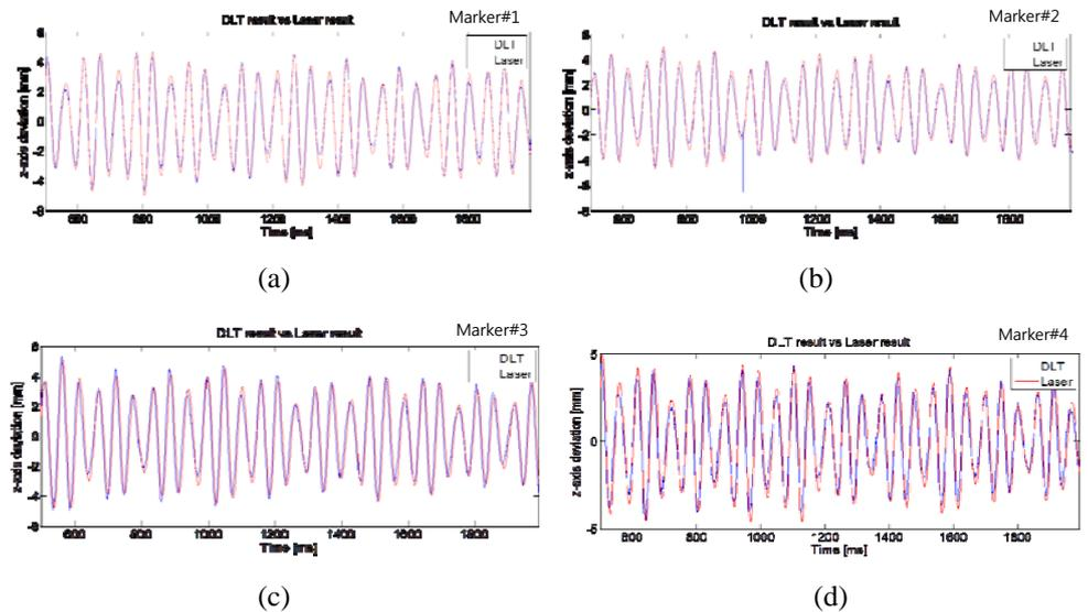
Fig. 5 Comparison of video-based measurement and laser measurement data: (a) marker#1, (b) marker#2, (c) marker#3, (d) marker#4
