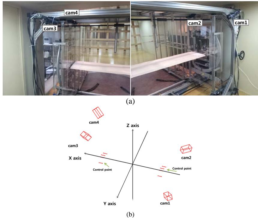
Fig. 4 Video-based measurement system: (a) camera position (b) camera calibration results
