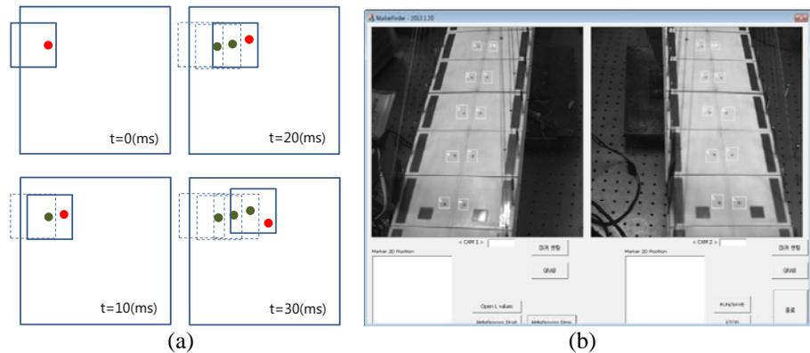
Fig. 2 Adaptive ROI algorithm; (a) traces of ROI and markers (b) snapshot of the user interface of the developed system
