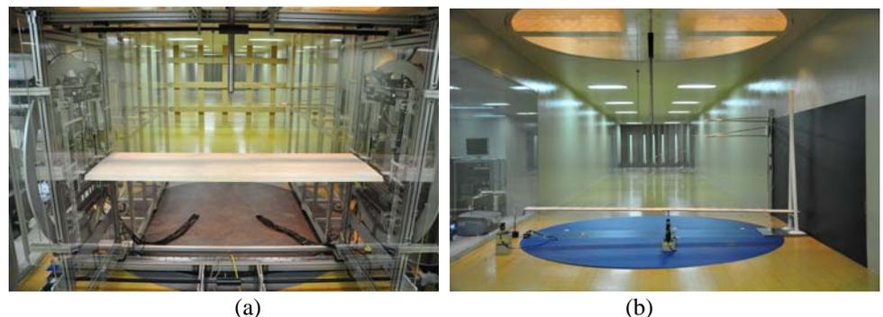
Fig. 3 Wind tunnel test setup: (a) bridge deck model connected to the spring support system (b) cable-stay bridge model
