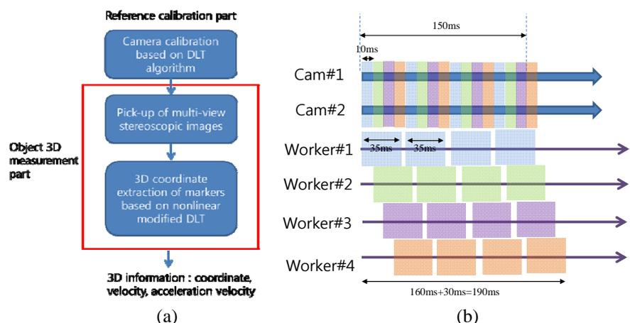
Fig. 1 DLT based real-time monitoring algorithm of 3D marker position trace; (a) work flow
