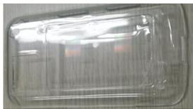
Fig. 1. Structural color of binary PMMA diffraction grating
