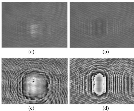
Fig. 5. Experimental results for holographic detection of off axis light beaming and focusing of light: (a) and (b) are captured images of the interference patterns of the off axis and focusing, respectively. And (c) and (d) correspond to extracted phase profiles.
