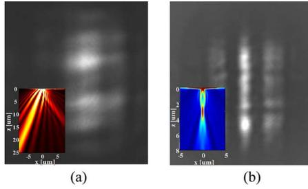
Fig. 2. Far-field views (in a plane parallel to metal surface) of the modified plasmonic light beaming fields captured by CCD: (a) off axis light beaming. (b) beam focusing. (Insets are numerically calculated  $x$ - $z$  plane results obtained by our rigorous coupled wave analysis technique.).
