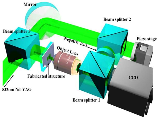
Fig. 4. Schematic of our off axis holographic microscopy setup.
