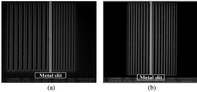
Fig. 3. SEM images of the fabricated beaming structures for: (a) off axis light beaming; (b) beam focusing. (The metal slit is located at the center of the grooves.).
