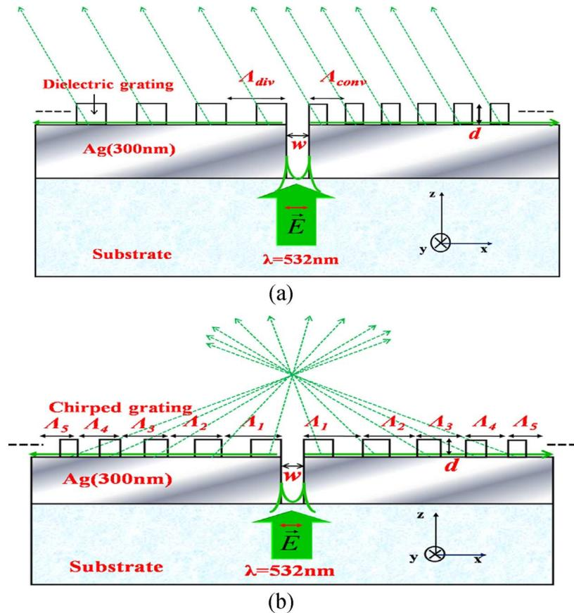
Fig. 1. Schematic of the manipulation of plasmonic light beaming using dielectric surface gratings circumventing the sub-wavelength metal slit: (a) off axis beaming structure; (b) beam focusing structure.
