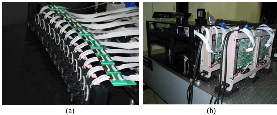
Fig. 11. Pictures of the dynamic holographic stereogram: (a) the curved array of SLMs mounted without upper arms and (b) whole system with electronic controllers.
