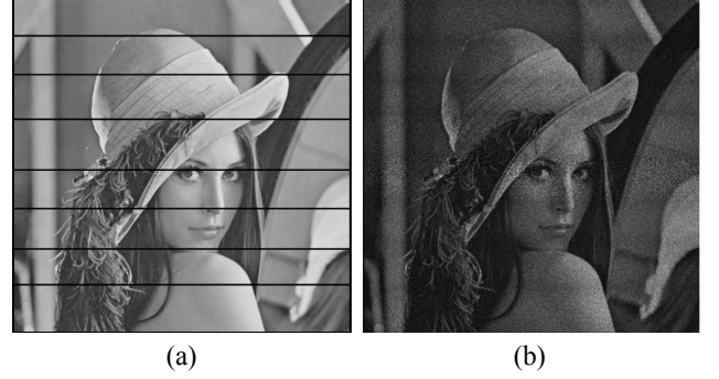
FIG. 4. (a) Segmentation of target image and (b) numerical reconstruction of binary holograms corresponding to each segmentation.
