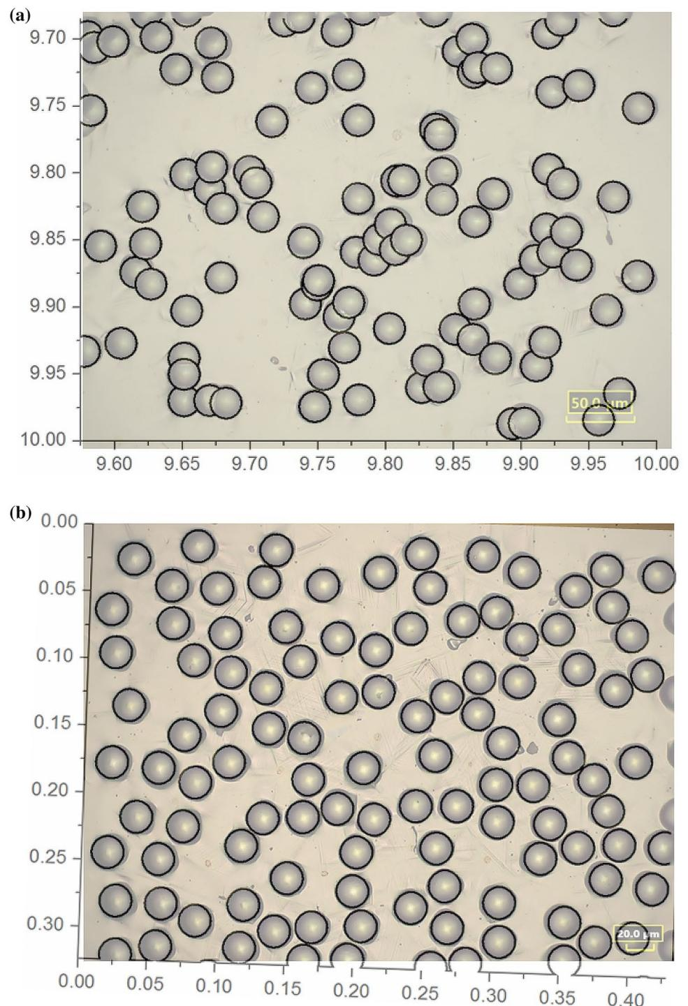
between the design of the microscale random patterns and the machined microscale random patterns on a metallic mold, the design results of Figs. 2 and 3 were overlaid on microscopic images of the machined mold, as shown in Fig. 8. The diameters and the coordinates were almost in perfect agreement in both the uncontrolled and controlled random patterns. These results meant that the microscale random patterns were machined with accurate positions
