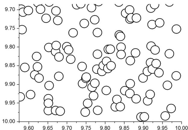
**Fig. 2** Coordinates of uncontrolled random pattern with diameter of 25  $\mu\text{m}$  and a fill-factor of 40% without consideration of the distance between each pattern
