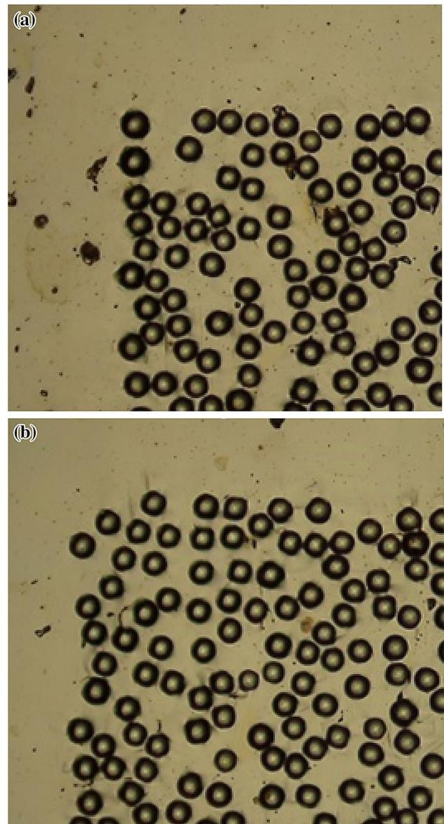
**Fig. 14** Comparison of machining results of **a** conventional coordinates and **b** new coordinates with a diameter of 25  $\mu\text{m}$  and a fill-factor of 40%
