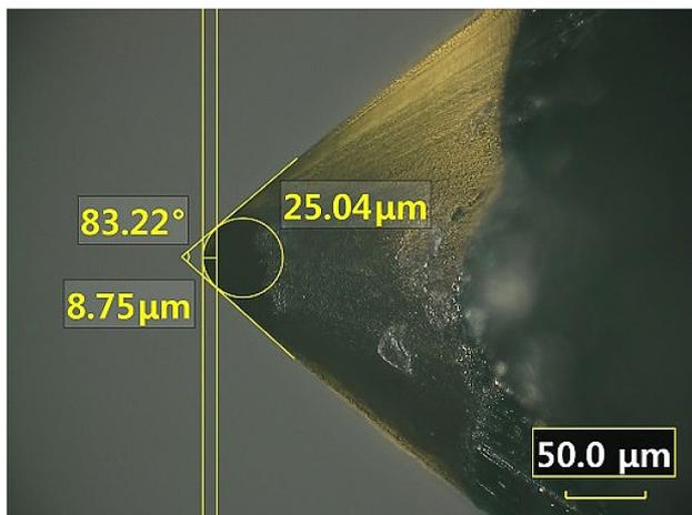
**Fig. 5** A machine tool with radius of 25  $\mu\text{m}$  for indentation machining
