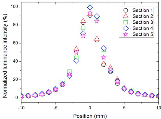
**Fig. 11** Comparison of the distributions of luminance of final spots measured at five different sections of one optical film having controlled random patterns
