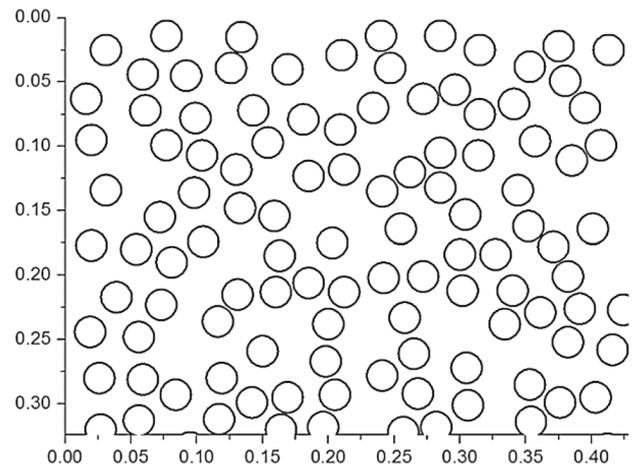
**Fig. 3** Coordinates of controlled random pattern with diameter of 25  $\mu\text{m}$  and a fill-factor of 40%, generated by the newly developed program in this study
