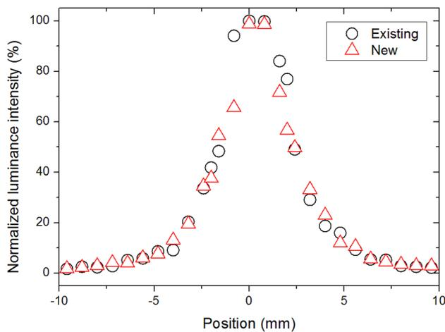
**Fig. 15** Comparison of two distributions of luminance of final spots conventional coordinates and new coordinates with the same diameter of 25  $\mu\text{m}$  and same fill-factor of 40%
