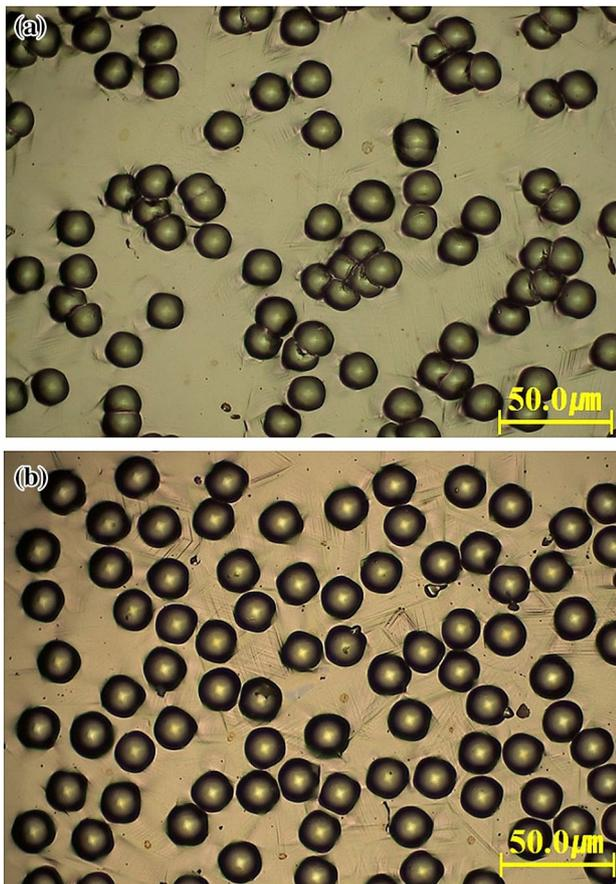
**Fig. 7** Machining results of **a** uncontrolled random patterns and **b** controlled random patterns (diameter of 25  $\mu\text{m}$  and a fill-factor of 40%)
