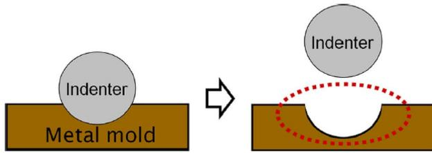
**Fig. 1** A novel indentation machining technology combining a dynamic indentation method and mechanical machining of a metal mold [18]
