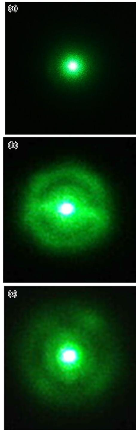
**Fig. 12** The shapes of final spots of laser light that has passed through optical films with **a** no pattern, **b** uncontrolled random pattern at Sect. 1 and **c** uncontrolled random pattern at Sect. 2
