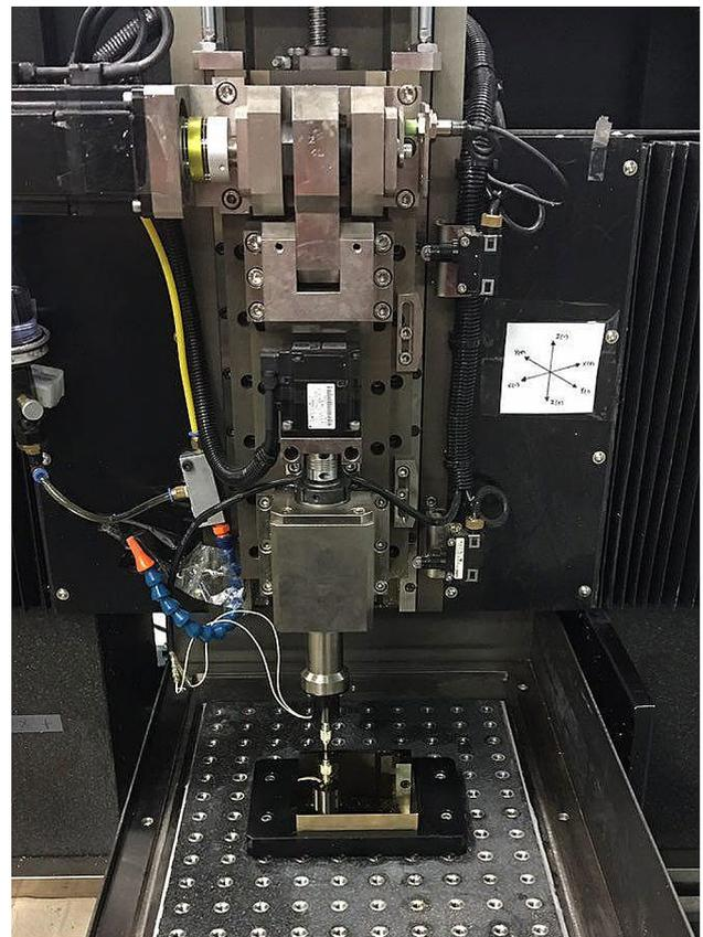
**Fig. 4** A dynamic indentation machining system used for precise planing and machining of microscale random patterns
