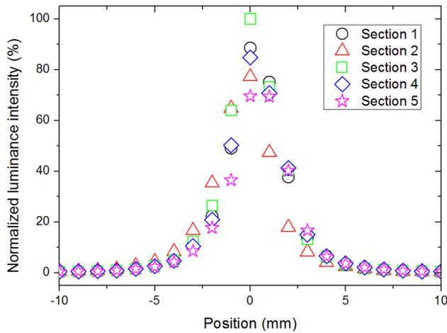
**Fig. 13** Comparison of the distributions of luminance of final spots measured at five different sections of one optical film with uncontrolled random patterns
