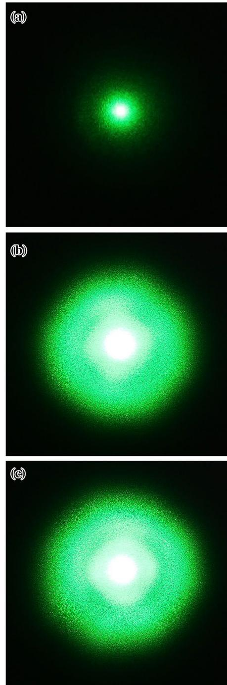
**Fig. 10** The shapes of final spots of laser light that had passed through optical films with **a** no pattern, **b** controlled random pattern Sect. 1 and **c** controlled random pattern at Sect. 2
