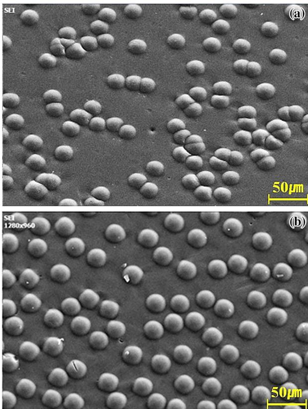
**Fig. 9** SEM images of the manufactured films with **a** uncontrolled random patterns and **b** controlled random patterns
