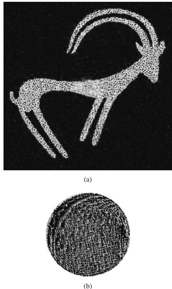
Fig. 1. (a) Diffraction image and (b) phase profile of conventional DOE without aperture apodization.
