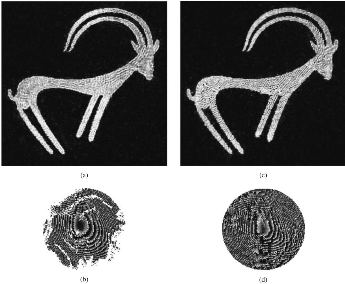
Fig. 3. (a) Diffraction image and (b) phase profile of DOE with apodized aperture, and (c) diffraction image and (d) phase profile of DOE designed by soft coding.
