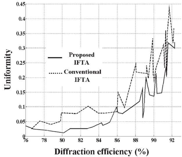
Fig. 1. Comparison of the performance of the conventional and the proposed IFTAs with respect to the trade-off between diffraction efficiency and uniformity. The number of iterations was 100 times for both the conventional and proposed IFTAs.
